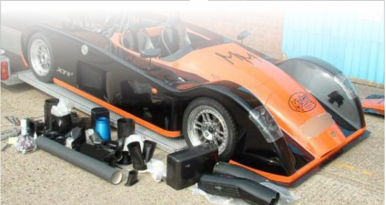
Height of air filter box can be customised to go under or fro more volume through the bonnet as shown
